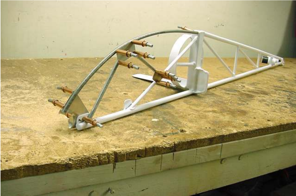
Building the right root rib.
